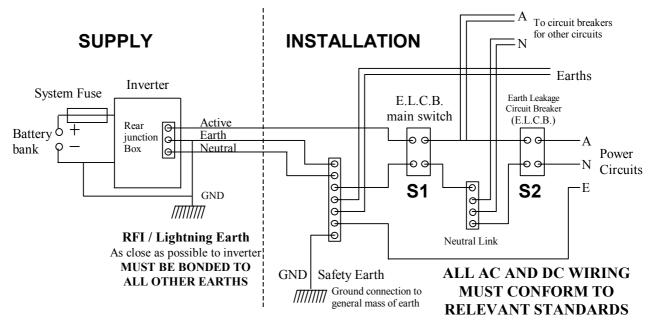
We suggest that you house your inverter along with other power generating equipment in a remotely sited purpose built area. Also make sure that the exhaust from your generator or other sources of heat or fumes are kept well away from the SA41. SEIAA (Solar Energy Industries Association Of Australia) installation guidelines must be followed.
